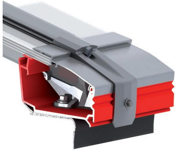
Material components that are perfectly coordinated with each other in the base profile of the continuous rooflight prevent fire from spreading on the roof if there is a fire inside the building – tested as per DIN 18234. Without any need for costly additional measures, such as gravel fill, the Linear Burn-through Protection prevents the “fuse effect” in the vicinity of the skylight opening thereby stopping the flames striking from inside and spreading to the roofing membrane.
