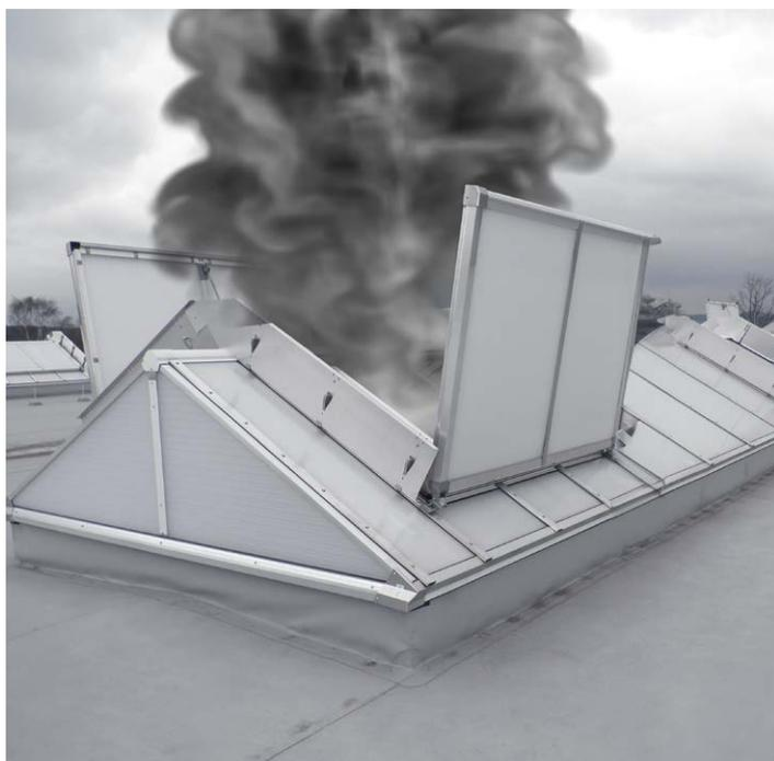
Our flap systems enable large-scale aerodynamic smoke extraction surfaces and large-scale full ventilation. Even with large dimensions, the flaps of the smoke lift prove to be an extremely stable overall system, even when open and under strong wind loads. In the event of a fire, they are opened quickly via thermal release or CO<sub>2</sub> or electrical remote release. If additional opening drives are used, our NSHEVs can be used for daily ventilation.
