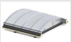
The smoke seal consists of an internal polycarbonate sheet and external aluminium plates. It is used for the compartmentalisation of fire sections whereby the polycarbonate of the Continuous Rooflight glazing melts and the smoke seal further restricts the fire section.
