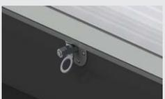
The anchor point for PPE is mounted on LAMILUX Continuous Rooflight frames prepared for such purposes and serves as an anchor point for personal protective equipment to prevent falls. It is an anchor point for using a carabiner in conjunction with a safety harness (EN 361) and fall arrest system (EN 363). No more than three persons are permitted to attach themselves to the rotatable anchorage eye.
