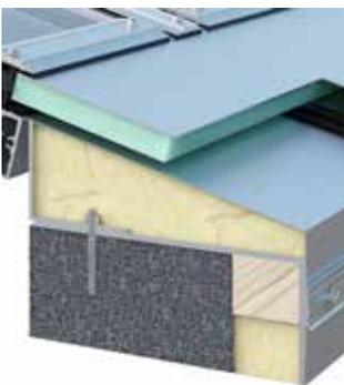
Installation on concrete upstand
